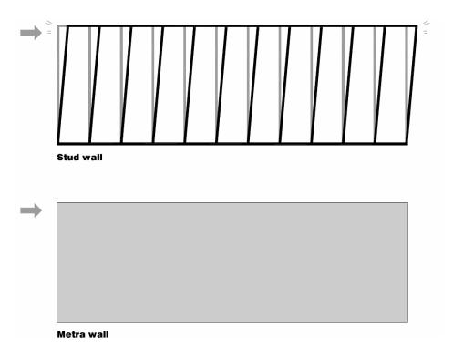
The Metrapanel system has inherent bracing capacity in all wall elements. Due to the high internal strength of Metra wall panels the bracing capacity is not limited by the wall panel itself.
